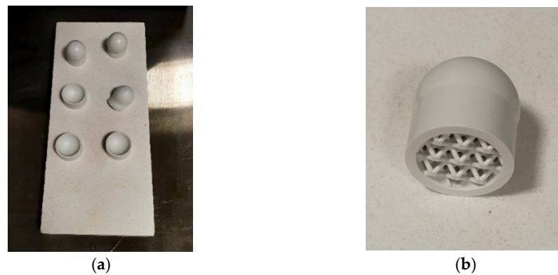
Figure 6. (a) Mushroom-type artifacts, down orientation, E support and WT = 2 mm. (b) Mushroom-type artifact, Up orientation, L support and WT = 2 mm.
