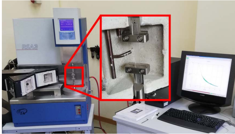
Figure 7. DMA RSA3 by T.A. Instruments. Test setup and clamp detail. Equipment at the University of Oviedo.
