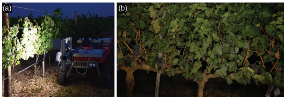
Figure 2. (a) On-the-go image acquisition with the multi-sensor mobile platform; and (b) image acquired with artificial illumination in which, due to appropriate illumination and camera parametrisation, the vines under evaluation are discernible from the darkened background.
